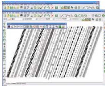
AutoLINE toolbar and sample linetypes are shown here running in AcceliCAD 2008, although Autodsys IntelliCAD and AutoCAD 2004–2009 are supported.
